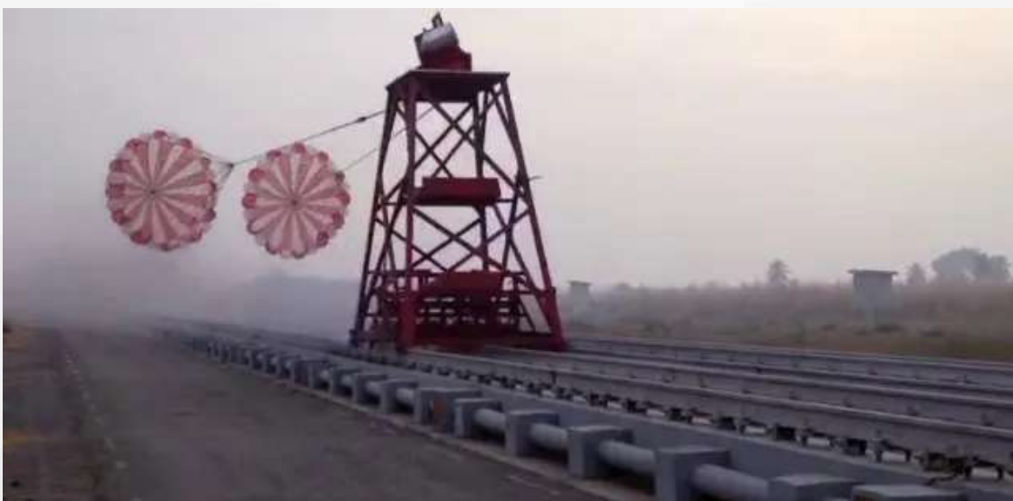
Description: Drogue Parachute Deployment Tests for Gaganyaan
